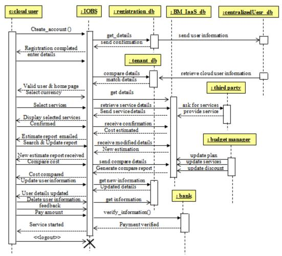
Figure 5. Sequence diagram of billing and metering Architecture for IaaS
