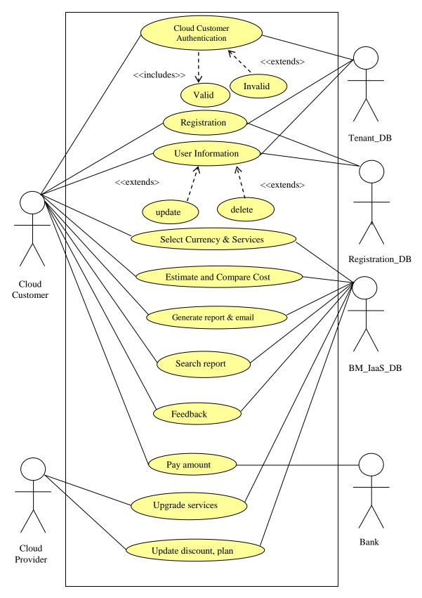
Figure 4. Use Case diagram of billing and metering Architecture for IaaS
