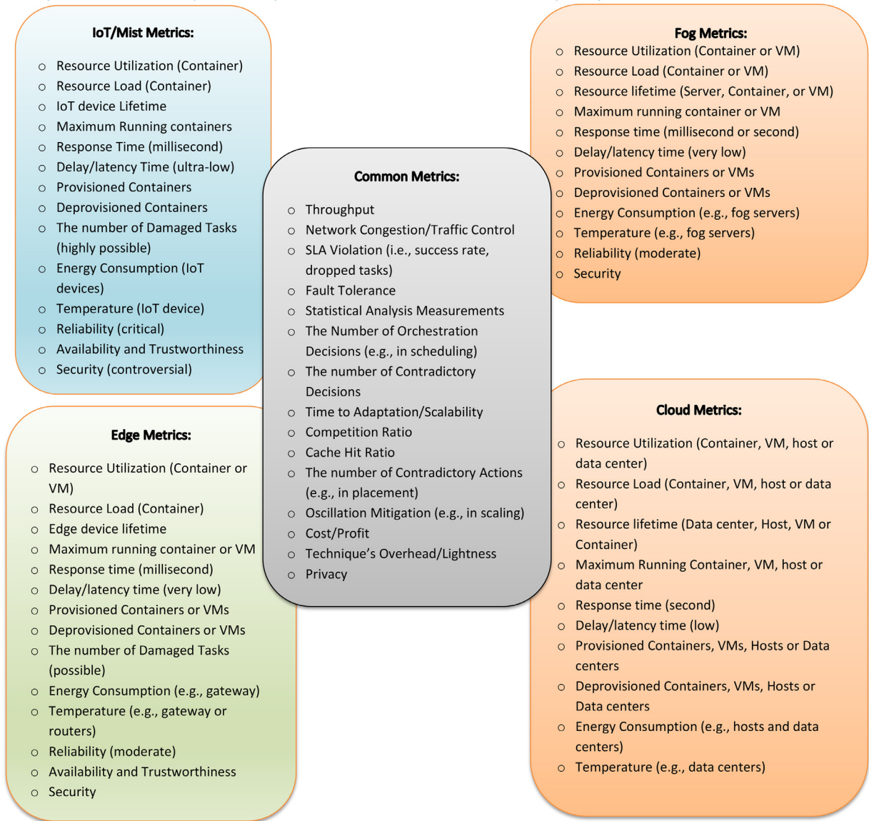
Fig. 2. A taxonomy of real-world performance metrics for evaluating IoT/Mist, Edge, Fog and Cloud Computing.
